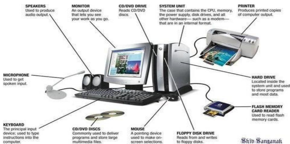
Fig 9.3.1: Components of a computer
